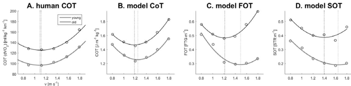
**Figure.** Human and model walking data. Walking data of young (gray) and elderly (black) adults are shown. The walking speeds of each minimum are marked with dotted lines. A. CoT of humans [1]. B. CoT of model. C. FoT of model calculated as square of muscle activations for walking distance,  $\frac{\sum \int A^2 dt}{d}$ . D. SoT of model calculated as square of normalized muscle forces,  $\frac{\sum \int \bar{F}^2 dt}{d}$ .
